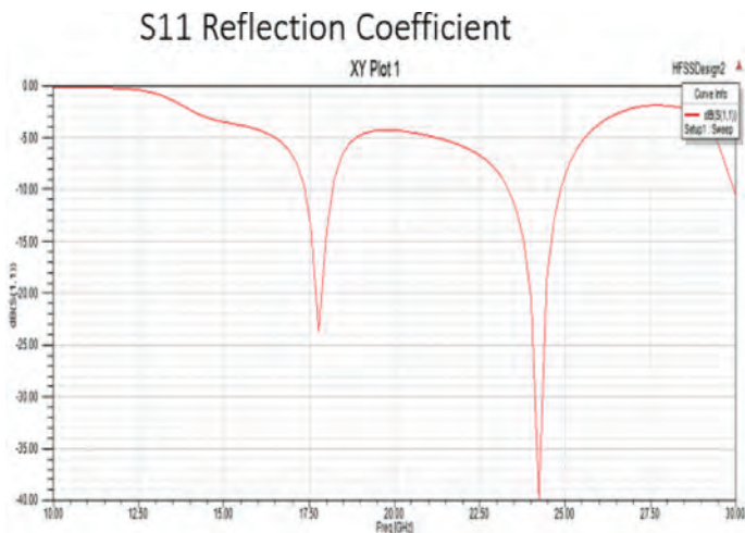
FIGURE 10.8 S_{11} of SIW horn antenna for millimeter wave frequency.
