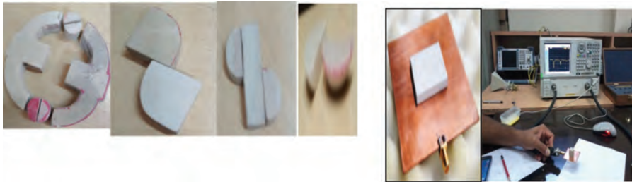
FIGURE 2.39 DRAs, fabrication stage to development, and then test and measurements.
