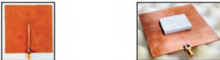
FIGURE 2.2 DRA fabricated with micro strip line.
