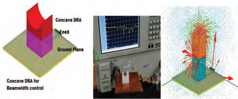
FIGURE A5.1 DRA concave shape with high permittivity on top material (narrow beam width, high directivity).
