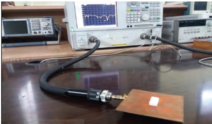
FIGURE A1.37 VNA measurement set up for s-parameters.
