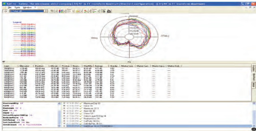
FIGURE 11.5 DRA device measured radiation pattern inside anechoic chamber.
