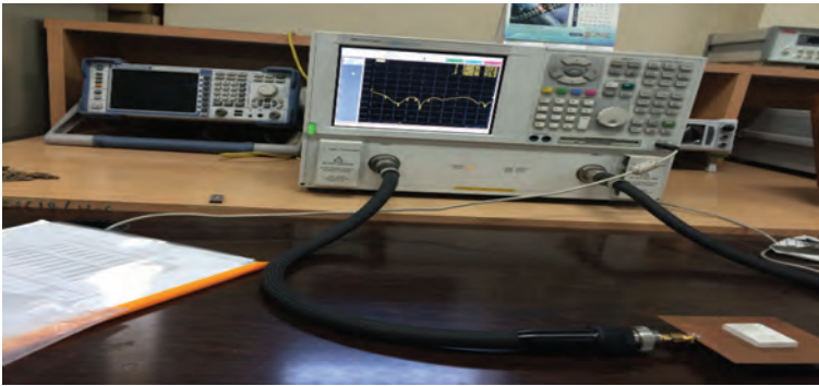
FIGURE 2.3 DRA measurements using VNA.
