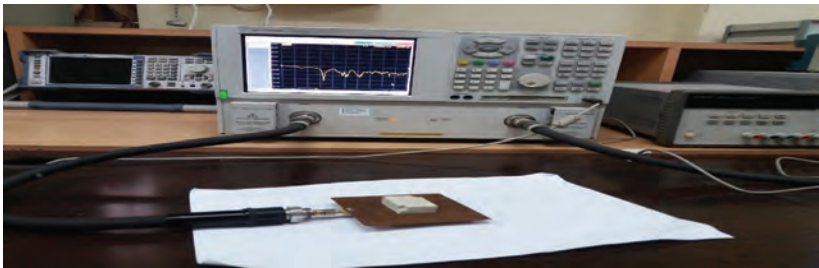
FIGURE A1.38 VNA measurement set up for s-parameters.
