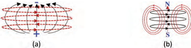
FIGURE 1.22 (a) Electric dipole and (b) magnetic dipole (solid line: electric field; dotted line: magnetic field).
