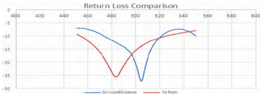
FIGURE 8.17 Reflection coefficients of NDRA at 483 and 502 THz with SiO 2 and Teflon substrates.
