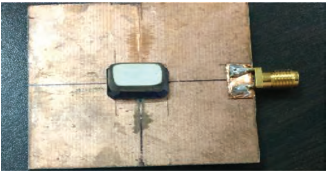
FIGURE 5.2 Sapphire antenna stacking with TMM.
