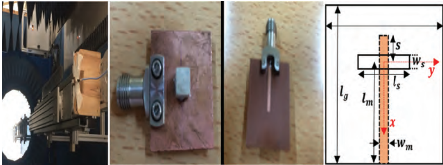
FIGURE 12.10 Long range vehicle radar rectangular DRA with wave launch connector (inside anechoic chamber measurement).
