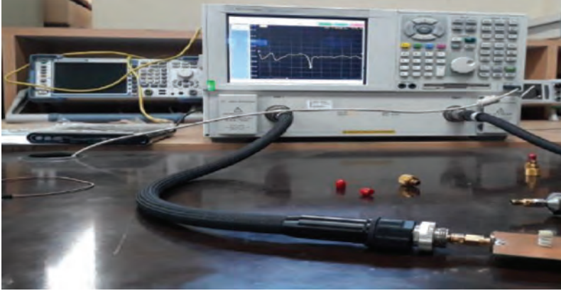
FIGURE A1.45 VNA measurement set up for s-parameters.
